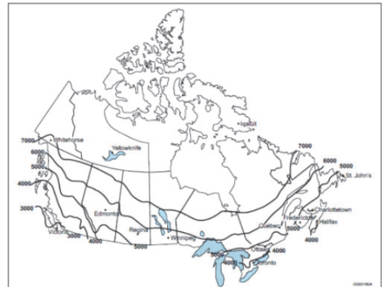
NECB 2017, Appendix Figure A-1.1.4.1.(1) – Contour Map of Approximate Annual Heating Degree Days
